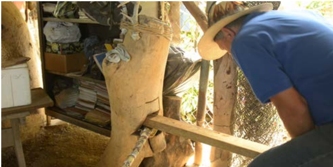
Figure 2: A “homemade” sugarcane press, called “chakki-chak”.
