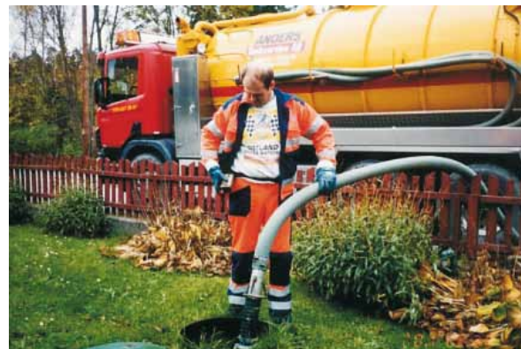
Figure 24: A conventional “Honey-sucker”, collecting sludge from on-site waste-water systems. Photo: Västerviks Municipality, Sweden
