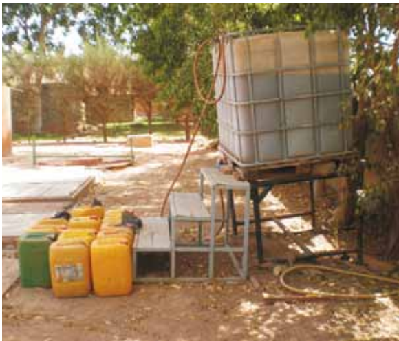
Figure 13: Storage of urine in one cubic metre tank.
